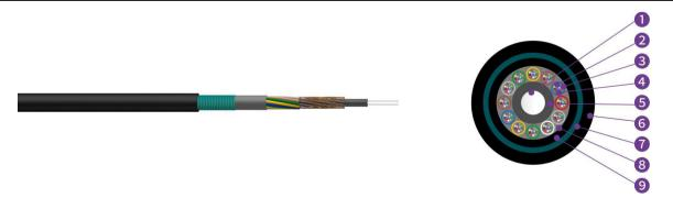
1,Strength Member 2,Fibre 3,Loose Tube 4,Tube Filling Compound 5,PE Layer 6,LSZH Sheath 7,PSP 8,Water Blocking Yarn 9,Fire Resistance Tape
