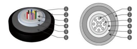
1, Fibers 2, PA Outer Sheath 3, Tube Filling Compound 4, Loose Tube 5, Glass fiber Yarn 6, LSZH Inner sheath
