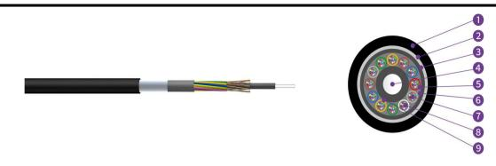
1,PE Outer Sheath 2,FRP Tape 3,PE Inner Sheath 4,Strength Member 5,Loose Tube 6,Cable Filling Compound 7,Fibre 8,Tube Filling Compound 9,PE Layer
