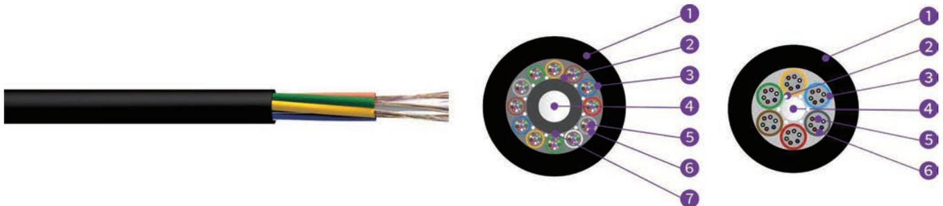
1, PE Sheath 2, Water Blocking Yarn 3, Loose Tube 4, Strength Member 5, Fibre 6, Tube Filling Compound
