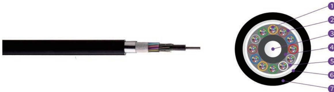
1.Fibers, 2.Loose Tube with Gel, 3.CSM, 4.PE Layer, 5.Compound, 6.Aluminum Tape, 7.PE Outer sheath
