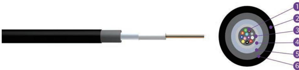
1, Fibers 2, PA Outer Sheath 3, Tube Filling Compound 4, Loose Tube 5, Glass fiber Yarn 6, LSZH Inner sheath
