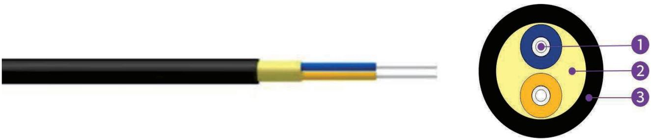
1, Tight Buffered Fibre    2, Aramid Yarn    3, Sheath
