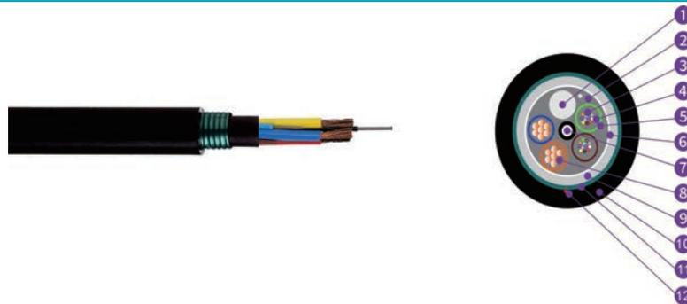
1, Filler 2, Cable Filling Compound 3, Fibre 4, Tube Filling Compound 5, Loose Tube 6, APL
