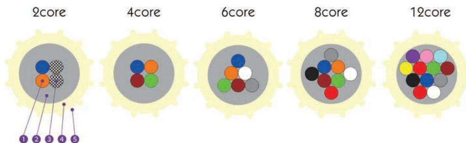
1,Optical Fibre    2,Resin    3,+2"Filled" Fibres    4, Low Friction Sheath    5, Groove
