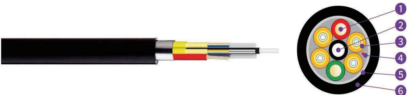
1, Copper Wire 2, Strength Member 3, Optical Sub-unit 4, Ripcord 5, APL 6, LSZH Sheath
