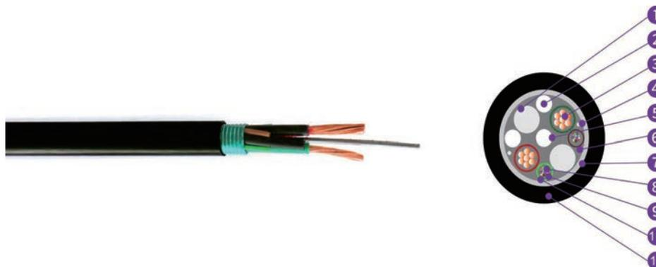
1, Filler 2, Filler 3, Copper Wire 4, Ripcord 5, Strength Member 6, Cable Filling Compound 7, APL 8, Fibre
