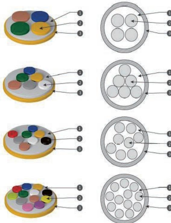
1, Resin    2, Fibress    3, Low Friction Groove Sheath
