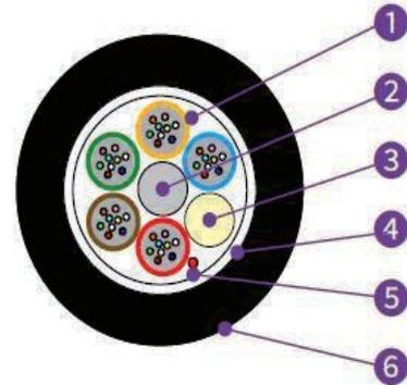
1. Loose Tube: thermoplastic material, containing optical fibers and filled with gel.
