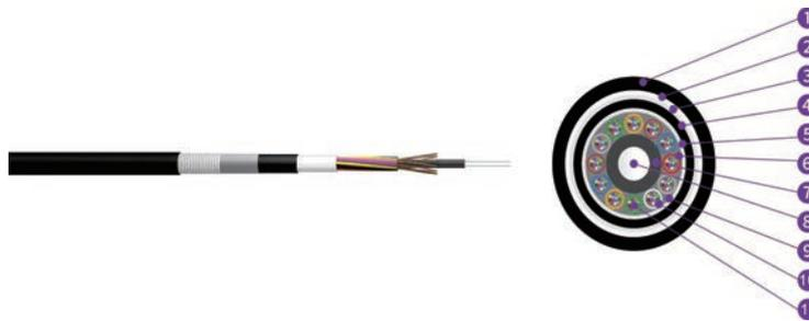
1, PE Sheath 2, Steel tape 3, Tube Filling Compound 4, PE Inner Sheath 5, APL 6, Loose Tube 7, PE Layer
