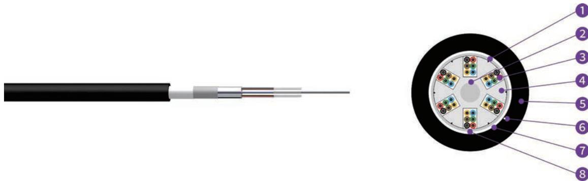
1, Rib Mark 2, Strength Member 3, Tight Buffered Fibre 4, Slot 5,Sheath 6,Ripcord 7,APL 8,Water Blocking Tape
