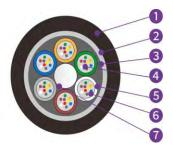
1,PE Sheath 2,Stainless Steel Tape 3,Cable Filling Compound 4,Fibre 5,Loose Tube 6,Tube Filling Compound 7,Central Strength Member
