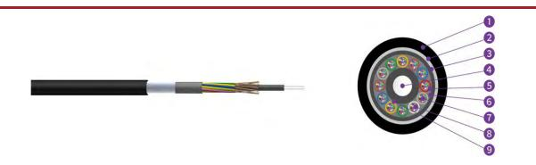
1,PE Outer Sheath 2,FRP Tape 3,PE Inner Sheath 4,Strength Member 5,Loose Tube 6,Cable Filling Compound 7,Fibre 8,Tube Filling Compound 9,PE Layer
