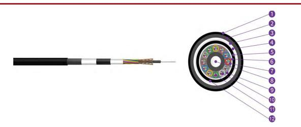
1,PA Outher Sheath 2,PE Middle Sheath 3,Stainless Steel Tape 4,Cable Filling Compound 5,PE Inner Sheath 6,APL 7,Loose Tube 8,Strength Member 9,Cable Filling Compound 10,Fibre 11,Tube Filling Compound 12,PE Layer
