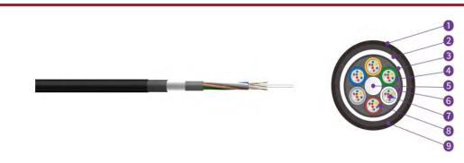
1,PE Outer Sheath 2,Flat FRP 3,PE Inner Sheath 4,Loose Tube 5,Strength Member 6,Cable Filling Compound 7,Fibre 8,Tube Filling Compound 9,Anti-rodent Middle Sheath
