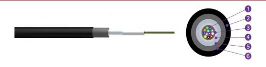
1, Fibers 2, PA Outer Sheath 3, Tube Filling Compound 4, Loose Tube 5, Glass fiber Yarn 6, LSZH Inner sheath
