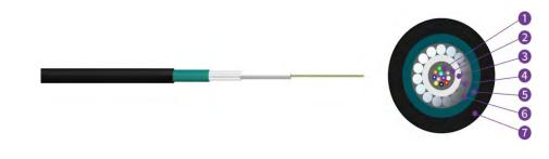
1, Fibers 2, Tube Filling Compound 3, Loose Tube 4, Steel wire 5, PSP 6, Cabling compound 7, PE Sheath
