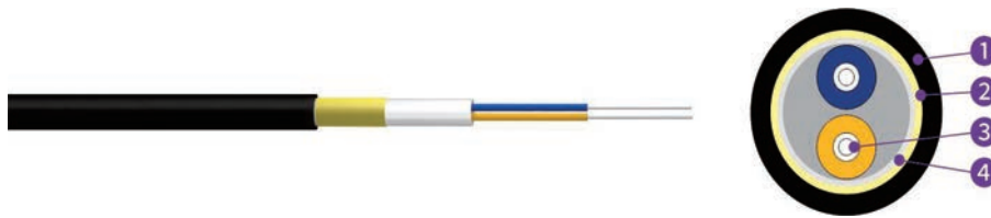
1,LSZH Sheath 2,Aramid Yarn 3,Tight Buffered Fibre 4,Helical Steel Hose
