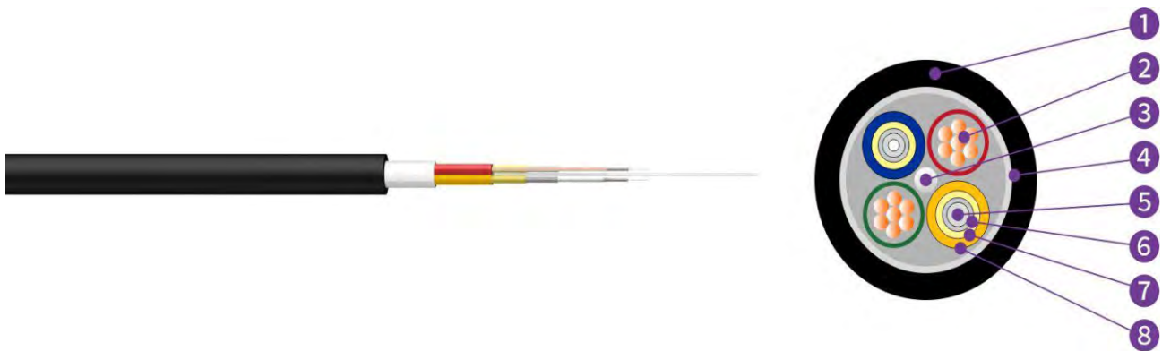
1,Outer Sheath 2,Copper Wire 3,Strength Member 4,Water Blocking Tape 5,Tight Buffered Fibre 6,Helical Steel Hose 7,Aramid Yarn 8,Sub-unit Sheath
