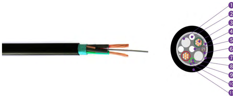
1, Filler 2, Filler 3, Copper Wire 4, Ripcord 5, Strength Member 6, Cable Filling Compound 7, APL 8, Fibre 9, Tube Filling Compound 10, Loose Tube 11, PE Sheath
