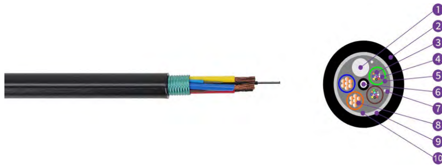
1, Filler 2, PE Sheath 3, Fibre 4, Tube Filling Compound 5, Loose Tube 6, Strength Member 7, Ripcord 8, Copper Wire 9, APL 10, Cable Filling Compound
